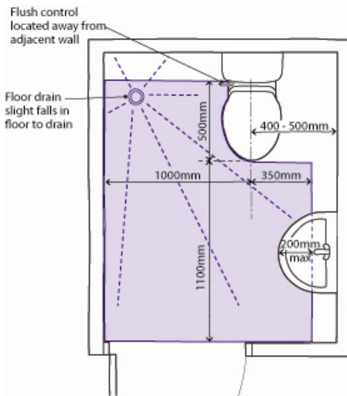
**Figure 10b - Example accessible WC compartment layout**
